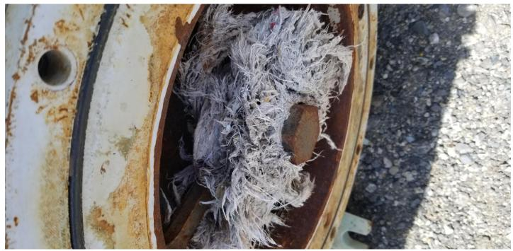
This picture is displaying an impeller from chopper pump responsible for mixing the digester tank at the wastewater treatment plant. This impeller was no longer able to mix the digester tank efficiently due to the numerous wipes wrapped around it. This is common on District equipment.
