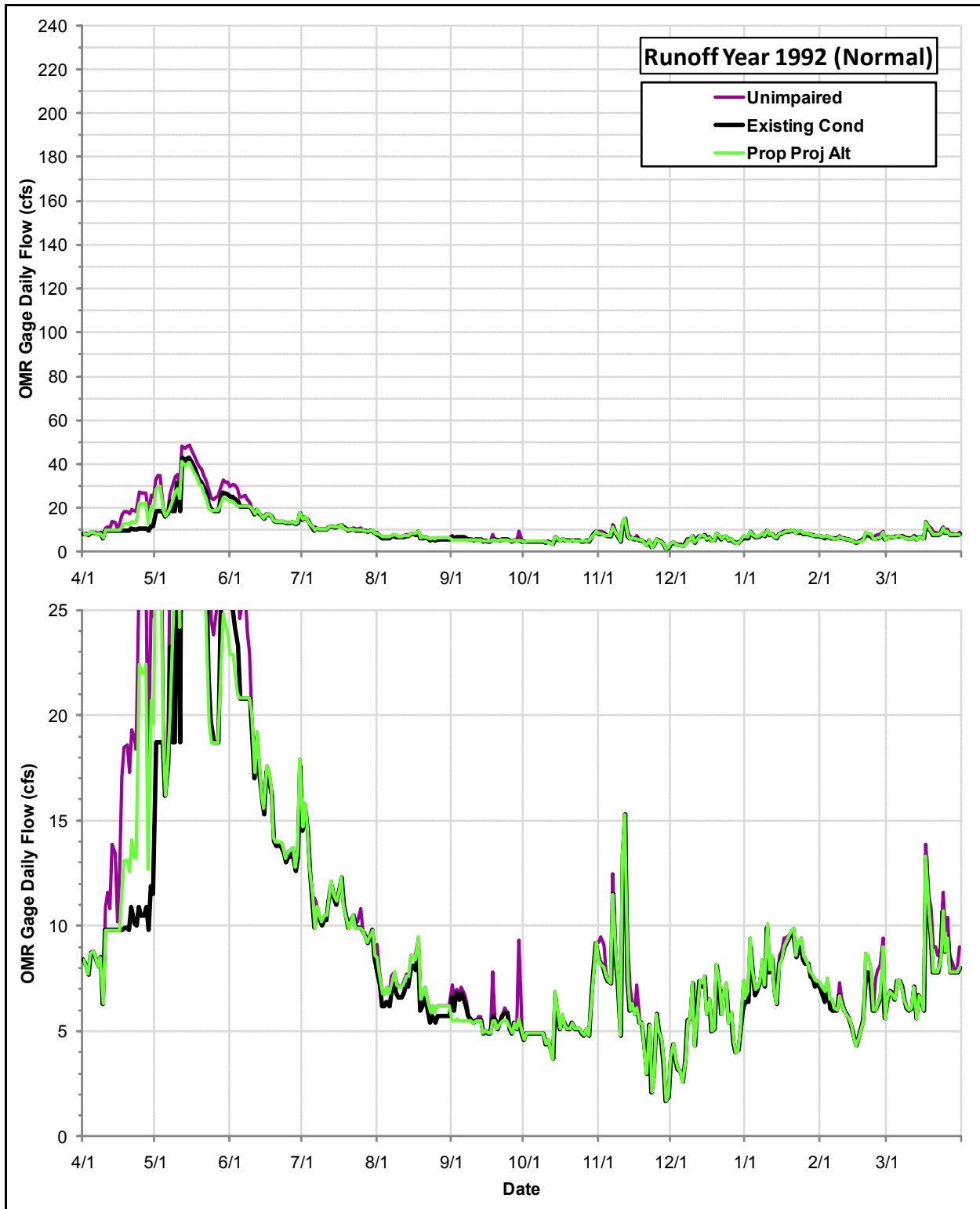
Daily Flows (cfs) at the OMR Gage under the Proposed Project Alternative, the Existing Condition and the Index Unimpaired Conditions during Runoff Year 1992
